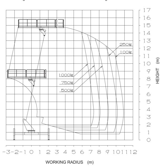
NOTE: Working ranges shown are for a case where aerial platform is set on a firm and level ground, and do not include boom deflection.
